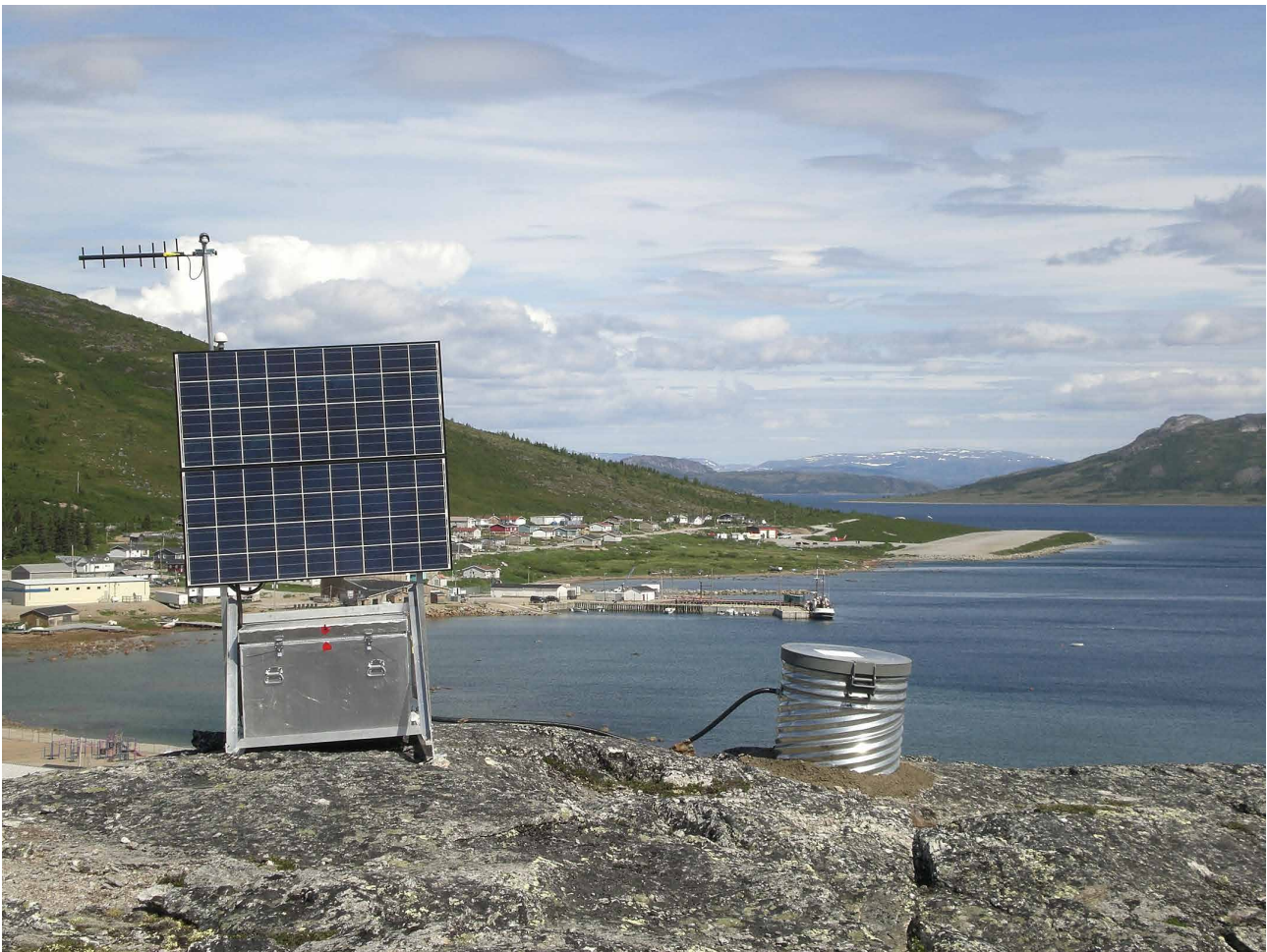
Seismograph station installed by Dr Darbyshire's team in Nain, Canada, in 2011.
